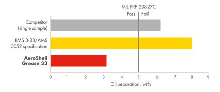
**CONTROLLED RELEASE.** AeroShell Grease 33 offers lower oil separation<sup>5</sup> to help for efficient lubrication throughout its life.
