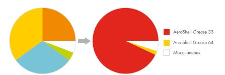
**MULTIPURPOSE PERFORMANCE.** Before AeroShell Grease 33 simplified maintenance, multiple greases were used on the Boeing 737 and other aircraft (left). Now AeroShell Grease 33 covers over 95% of application points. With its partner AeroShell Grease 64, an extreme-pressure grease, over 98% of application points are covered (right).
