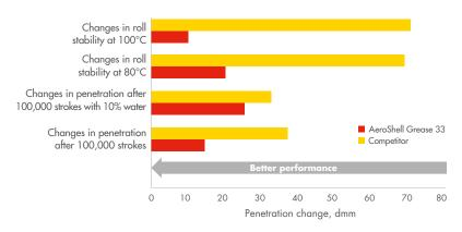
**STAYING WHERE YOU NEED IT.** AeroShell Grease 33 offers superior mechanical stability after being worked in two ways and when mixed with 10% water.<sup>4</sup>
